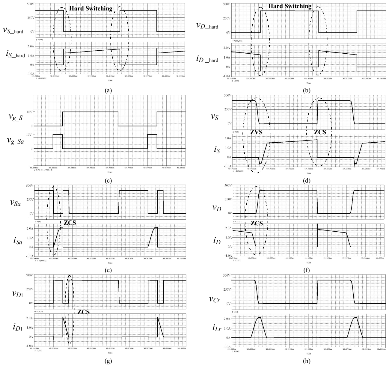
Figure 7. Simulation results of the proposed converter (a) Voltage and current of S under hard-switching condition (b) Voltage and current of D under hard-switching condition (c) Turn on signal of S and S_a (d) Voltage and current of S (e) Voltage and current of S_a (f) Voltage and current of D (g) Voltage and current of D_i (h) Voltage of C_r and current of L_r .
