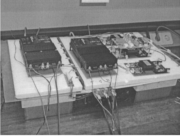
Fig. 7. Three-phase converter with PEBB.
